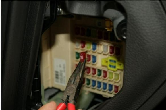
Please connect red power cable into the fuse as shown below in the picture.
