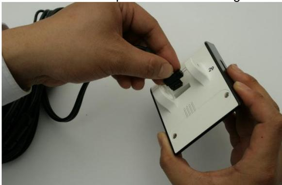
Please insert the supplied SD card into Plug 'n' Go Drive unit. If inserted correctly the SD card will click and lock in the recess.
