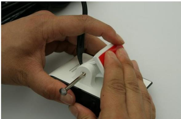
Connect the bolt and find a suitable position on the wind screen before peeling the red sticker off the mounting holder. Ensure power cable is not obstructing the camera view. Bolt can be loosen to adjust the Plug 'n' Go Drive.
