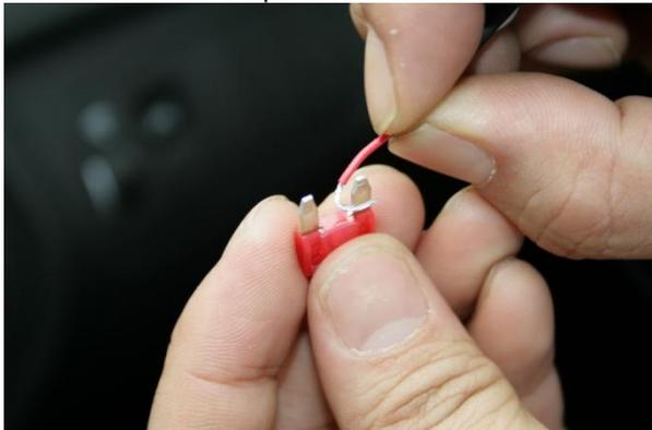
After connecting the red cable into the fuse, please re-connect the fuse into the original location as below picture shows.
